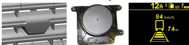
The driver sets a desired cruise speed and following distance mode to a vehicle ahead. If necessary ACC will adapt the vehicle speed to maintain the preset following distance.
